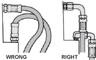
Use elbows and adapters to relieve strain and allow neater installations for easier accessibility and maintenance
