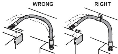
Hose movement in 2 planes can induce twist. A clamp at the nodal point will avoid the need for a swivel
