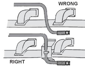
Avoid hot manifolds etc where possible, or isolate with fire sleeve or other protective means
