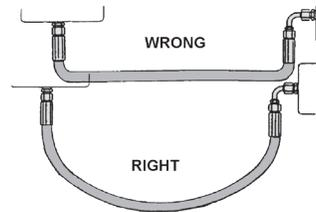
Using too small a bend radius will greatly reduce hose life, and may cause line collapse and flow restriction
