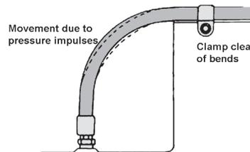
Avoid restricting hose movement around bends. Clamping should occur away from the area of movement
