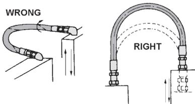
Ensure that bending of a hose occurs in the same plane as the movement of the attachment point to avoid induced twist
