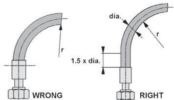
Have a straight section before bending commences. Use a PIRTEK Hose Guard on large multi-spiral hoses to assist
