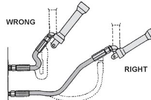
Remember that the metal hose fittings are not part of the flexible portion. Allow ample free length for flexing
