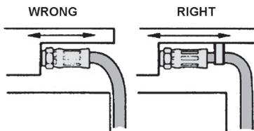
Use clamps to support long runs or keep hose away from moving parts. Clamps mustn't be allowed to move (abrasion)
